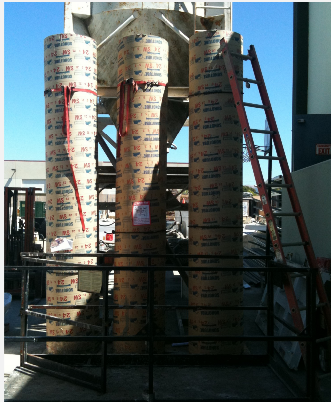
Performing the 10' Sonotubes Stable Flow tests on-site
